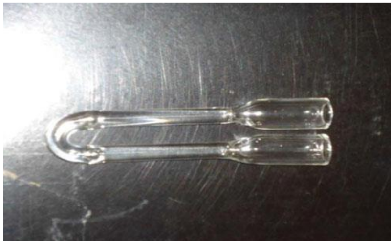
Figure 1. Experimentally designed Pyknometer.
